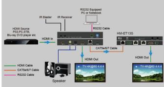
HB-102A HB-104A HB-108A is a highquality, longreach 4K@60Hz (4:4:4) HDBaseT distributor that takes one longreach HDBaseT input, equalizes and reclocks the signal and distributes it to two identical HDBaseT outputs. The VM2DT distributes native longreach HDBaseT signals with up to 4K video resolution, along with their reextension over longreach HDBaseT to feature an integrated extender distributor product
